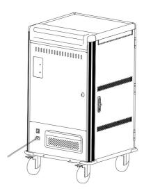
5. Turn on the power switch to start charging ,the led indicates red color to show the device in charging ,then the device full charged, the led turn to green color .
